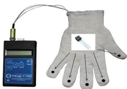
Figure 2. The model of a thermometric glove.
